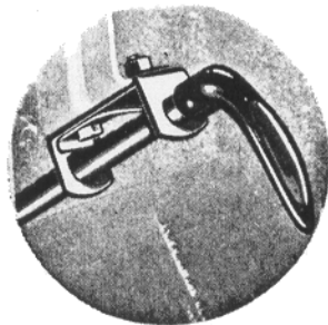
The Overland hand brake lever is located under the dash at the left of the driver.
