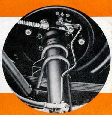
• The Hydraulic Brakes are oversize. Designed to give equal action on all four wheels, they also provide an extra margin of braking power with only 17 pounds of car weight to every square inch of brake surface. Brake drums are composite cast alloy iron for long life and easy action.
