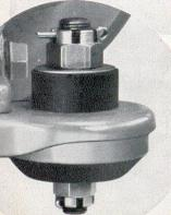
• The engine is floated upon four live rubber mountings. The engine is smooth at all speeds.
