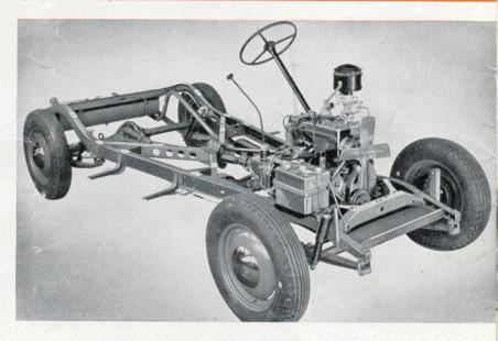
• Willys-Overland engineers are particularly proud of this sturdy, modern chassis. Every principle and detail have been engineered to offer dependable performance and long life in the new Overland. The engine is mounted low in the chassis for a low center of gravity. The front and rear springs are carefully engineered to provide a smooth, level ride. The semi-floating rear axle is over-size and sturdy.
