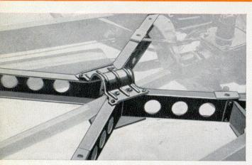
● The rugged frame with K-X cross members and heavy gauge steel double-drop construction offers strength in excess of needs. All parts designed to provide greater safety.
