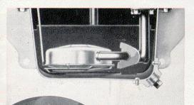
• The Float-O oil intake prevents sludge, water and dirt from getting into the oil circulation system.
